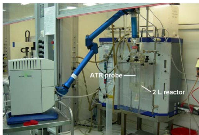
Figure 6.11. The platform used for scale-up studies ( T = 343 K, methanol/EC = 4, 10 wt.% (10g) catalyst).
