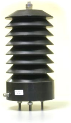
Figure 13 MV Dimat CAMT capacitive coupling unit used in the measurements
