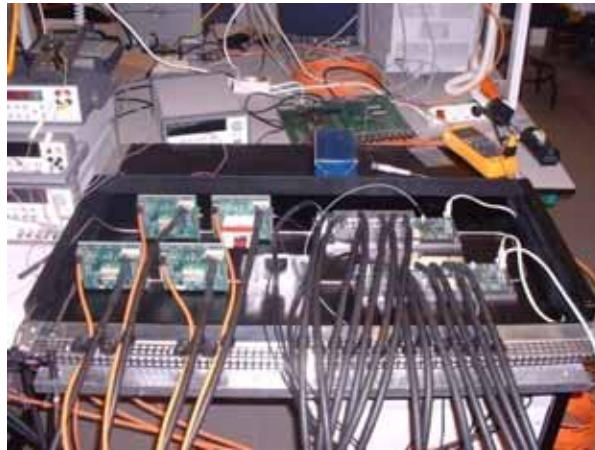
Figure 104. View of the box used at laboratory for stability and cooling tests
