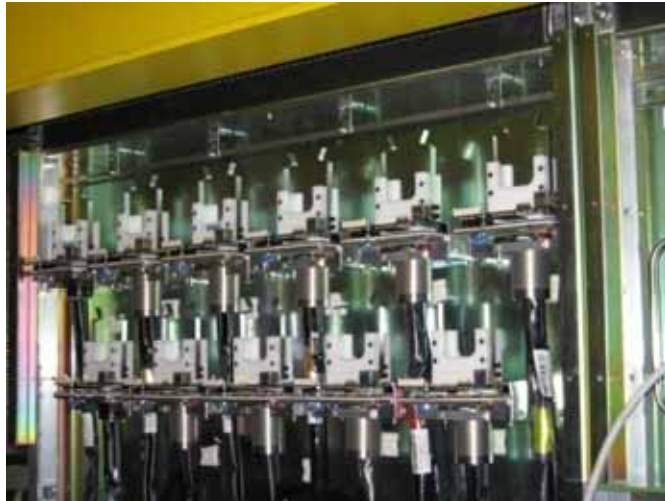
Figure 111. Box of 11 VFE Units without cabling
