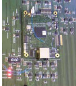
Figura 2.45. SPECS mezzanine resident a la CB.
