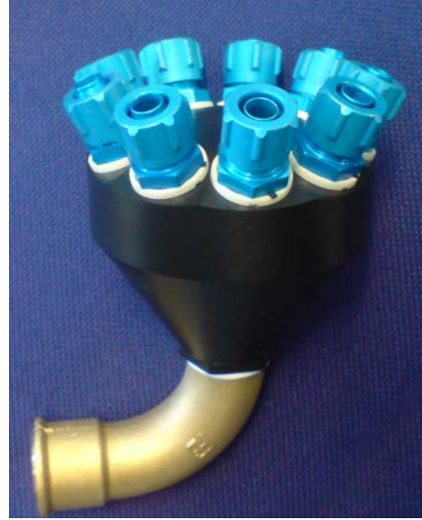
Figure 4.3: Manifold to split the main liquid flow into 9 lines
