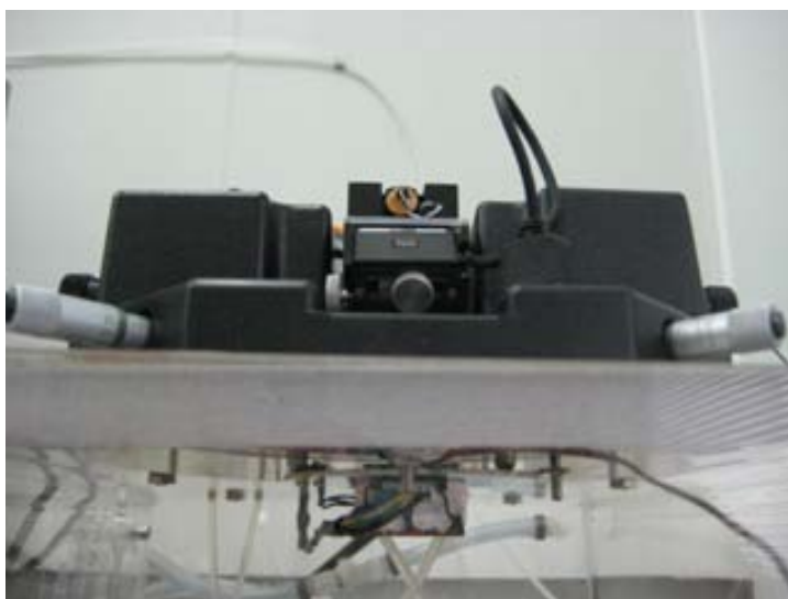
Figure 2.7: The scanner electronics (top part) is separated from the cantilever, sample and sample holder (lower part) by the glove box. While the sample stage and the cantilever are in the controlled humidity conditions the electronics remain outside the glove box. In the rear part the inlet of the N 2 gas can be seen.
