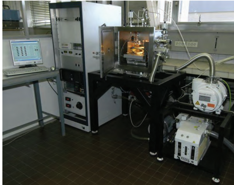
Figure A.1: Photograph of the HWCVD deposition system used in the framework of this thesis.
